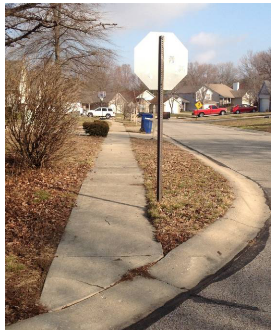
Example of signage protrusion
